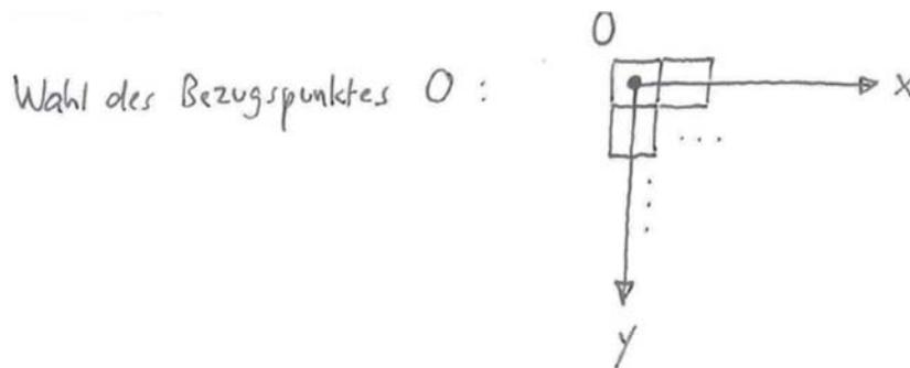
$$\sum_i (m_i \vec{r}_i) = m \cdot \vec{r}_S \quad \left| \begin{array}{l} m_i = \text{konst.} =: m_0 \\ : m \end{array} \right.$$
