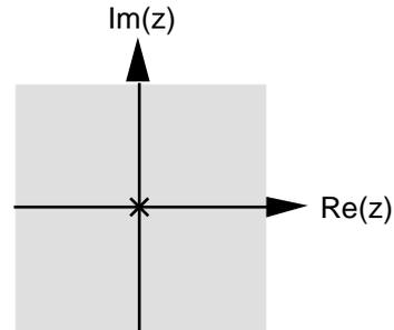
$$e) \quad X(z) = -\frac{3}{2} \frac{z^{-1}}{\left(1 - \frac{1}{2}z^{-1}\right)(1-2z^{-1})} = -\frac{3}{2} \frac{z}{\left(z - \frac{1}{2}\right)(z-2)} \quad \frac{1}{2} < |z| < 2$$
