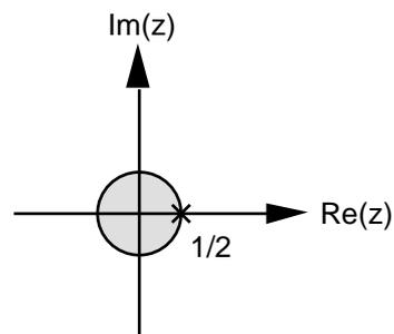
$$d) \quad X(z) = \frac{1-(2z)^{-10}}{1-(2z)^{-1}} \quad \left( \begin{array}{l} |z| > 0 \\ z = \frac{1}{2} \end{array} \right) = \frac{z^{10} \cdot \left(\frac{1}{2}\right)^{10}}{z^9 \left(z - \frac{1}{2}\right)} \quad \left( \begin{array}{l} |z| > 0 \\ z = \frac{1}{2} \end{array} \right)$$
