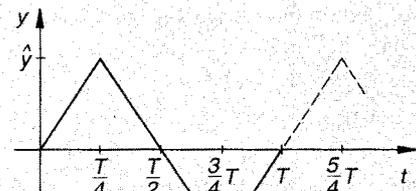
$$y(t) = \frac{8\hat{y}}{\pi^2} \left( \frac{1}{1^2} \cdot \sin(\omega_0 t) - \frac{1}{3^2} \cdot \sin(3\omega_0 t) + \frac{1}{5^2} \cdot \sin(5\omega_0 t) - + \dots \right)$$
