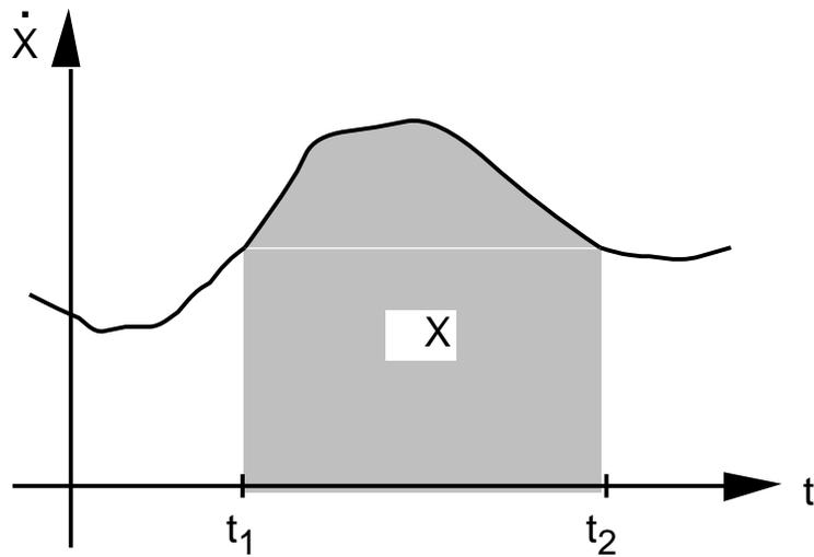
$$X = X(t_2) - X(t_1) = \int_{t_1}^{t_2} \dot{X}(t) dt$$
