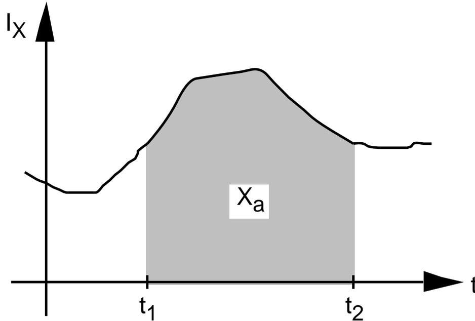
$$X_a = \int_{t_1}^{t_2} I_X(t) dt$$
